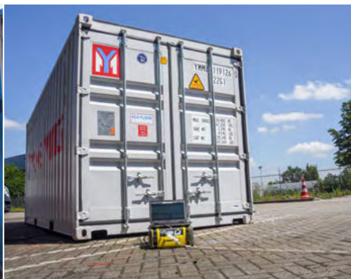
Meting van de gasconcentraties met de Gasmet FTIR. (© Customs Support Safety)
